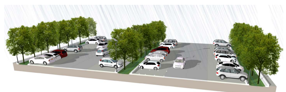
Bioswales are integrated in all surface parking lots throughout RiverBend.
