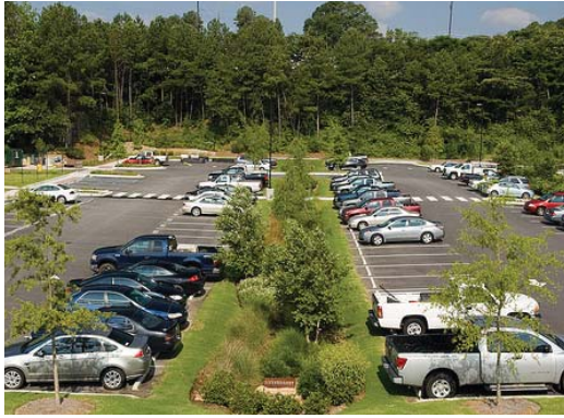
Image 55: Example of parking lot Bioswale
