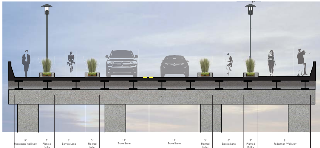
Image 29: Long-term complete street design for Tift Street Bridge
